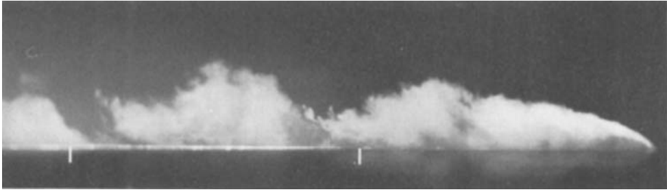
FIGURE 12. Instantaneous smoke flow visualization on model centreline ( Z = 0 ). Flow from right to left. Marks indicate X/L_R = 1.0 and X/L_R = 2.0 . Re_D \approx 3.2 \times 10^4 .
